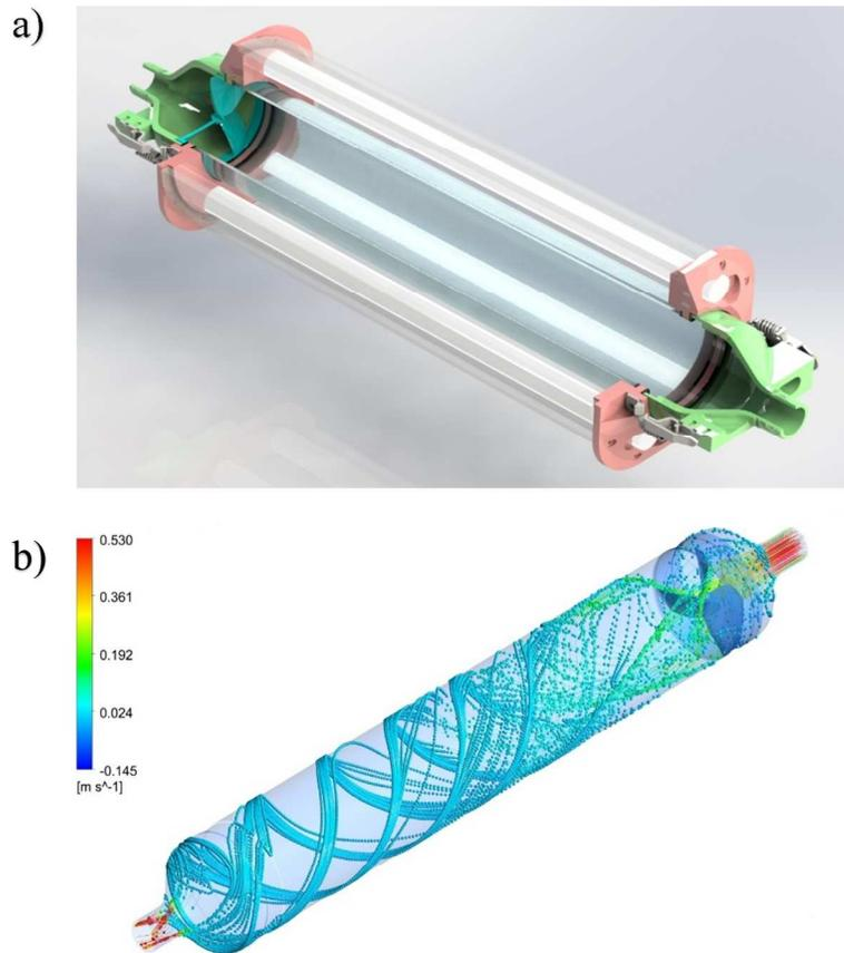
**Figure 1.** Isometric view (a) and particle tracking through the UV system (b).
