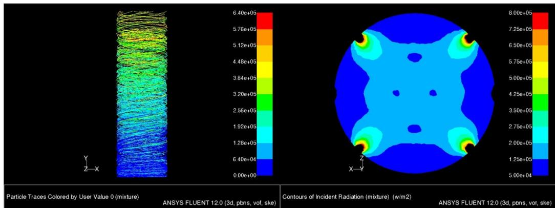
Figure 2: Computer simulations of the patterns of flow within the quartz cylinder (left) and of the UV intensity produced within the water column due to 4 UV lamps (right).
