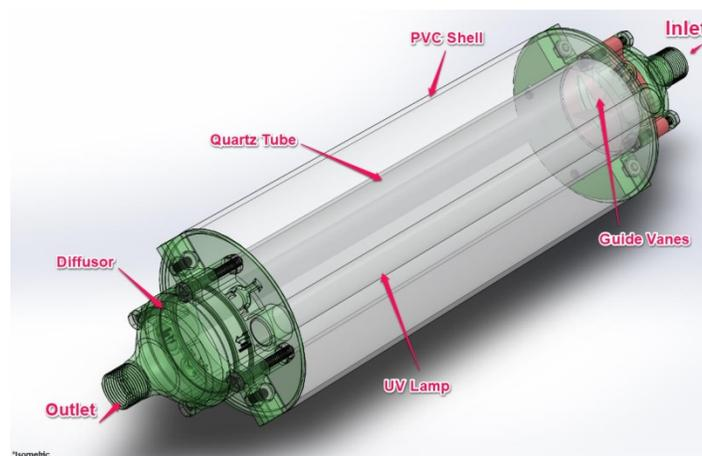
Figure 4: Schematic drawing showing the main components of the developed point-of-use UV system.
