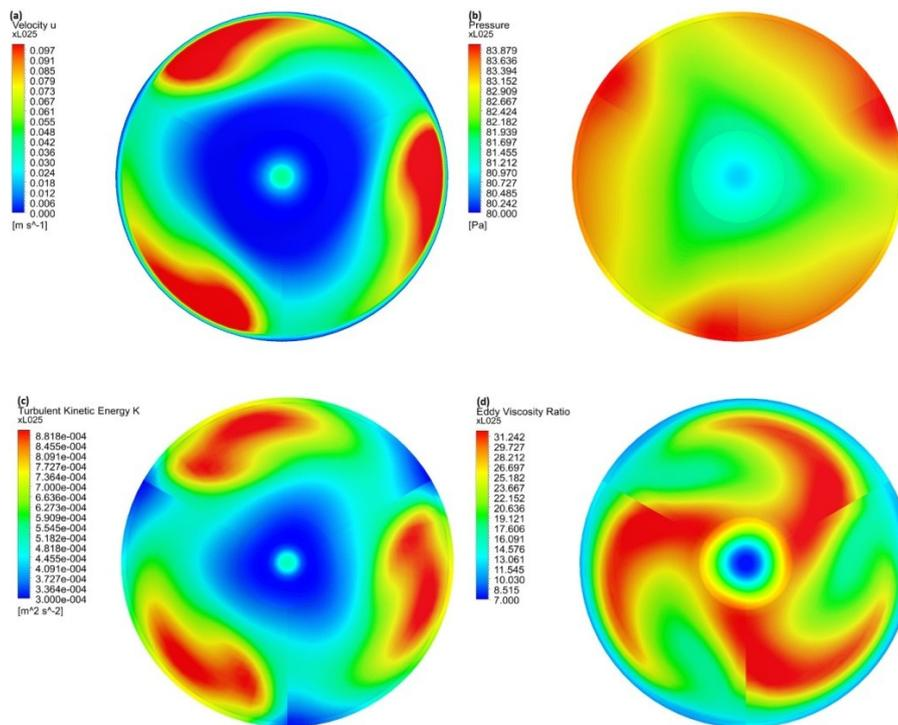
**Figure 5.** Predicted cross-sectional contours of the mean axial velocity (a), the static pressure (b), the turbulent kinetic energy (c), and the ratio of turbulent to molecular viscosity (d). The enhanced levels of turbulence kinetic energy and thus of turbulent mixing due to swirl are evident.
