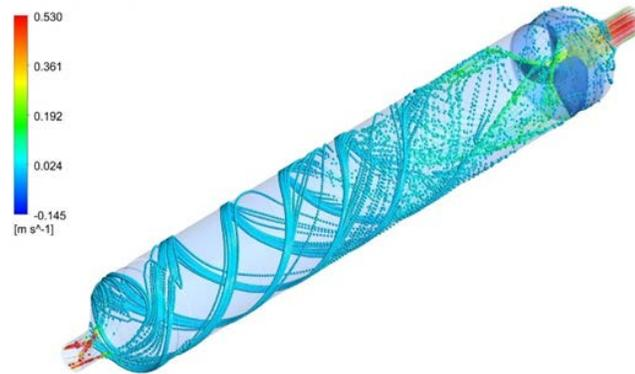
Figure 5: Computer simulations showing the helical trajectories of massless particles that enter the system to be exposed to UV light.
