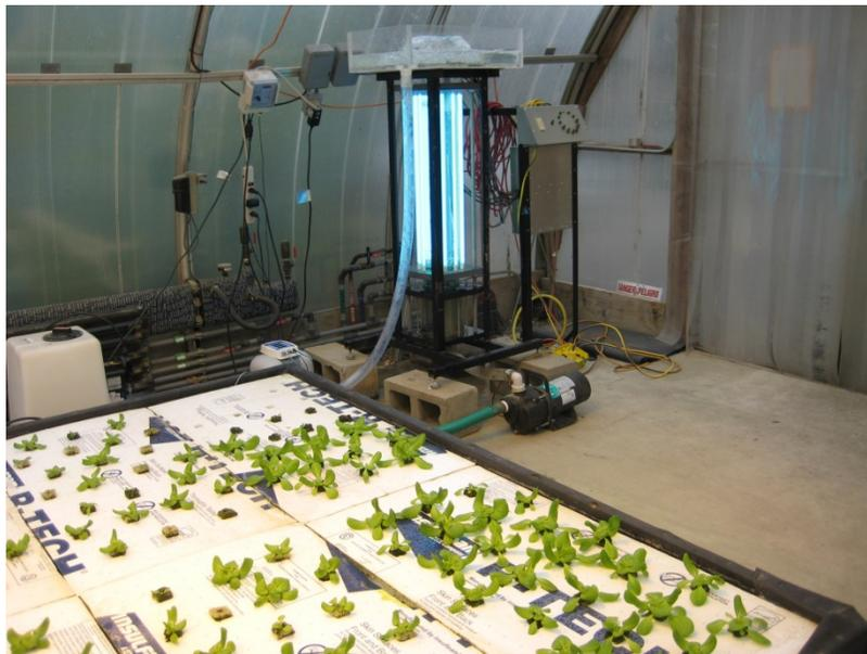
Figure 3: The UV vortex reactor in operation at the UCD experimental greenhouse.
