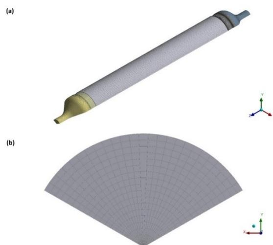
**Figure 2.** The computational grid used for the computer simulations. View along the side of the system showing the overall arrangement (a), and a cross-sectional view of the grid distribution in a sector (b).
