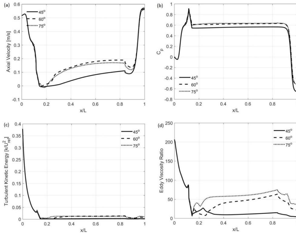
**Figure 4.** Predicted variation along the reactor centerline of the mean axial mean velocity (a), the pressure coefficient (b), the turbulence kinetic energy (c), and the eddy-viscosity ratio (d). Results are plotted for three different values of blade pitch.
