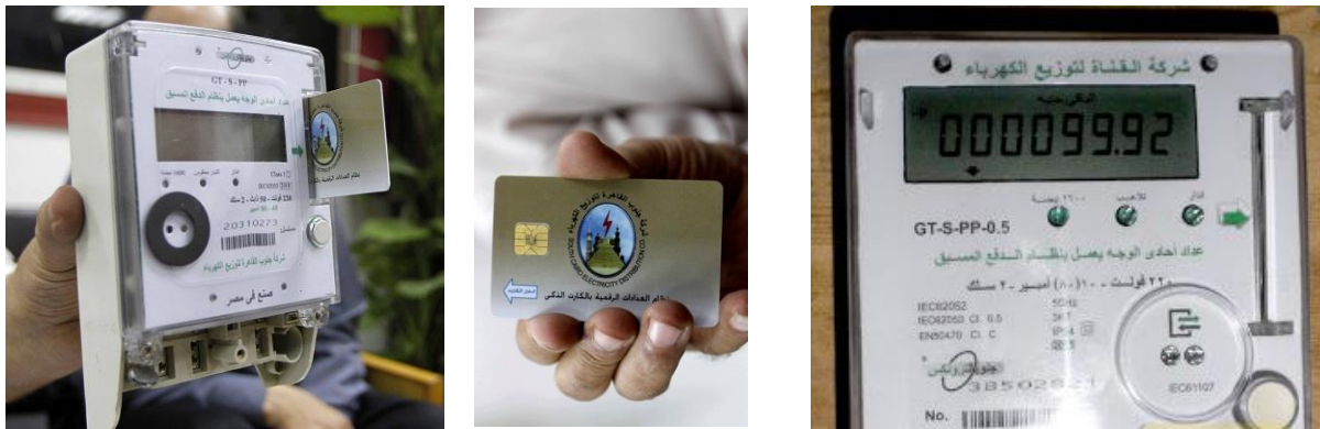
Figure 26: Prepaid Electricity Meters Distributed to Residents of Sheikh Zayed
