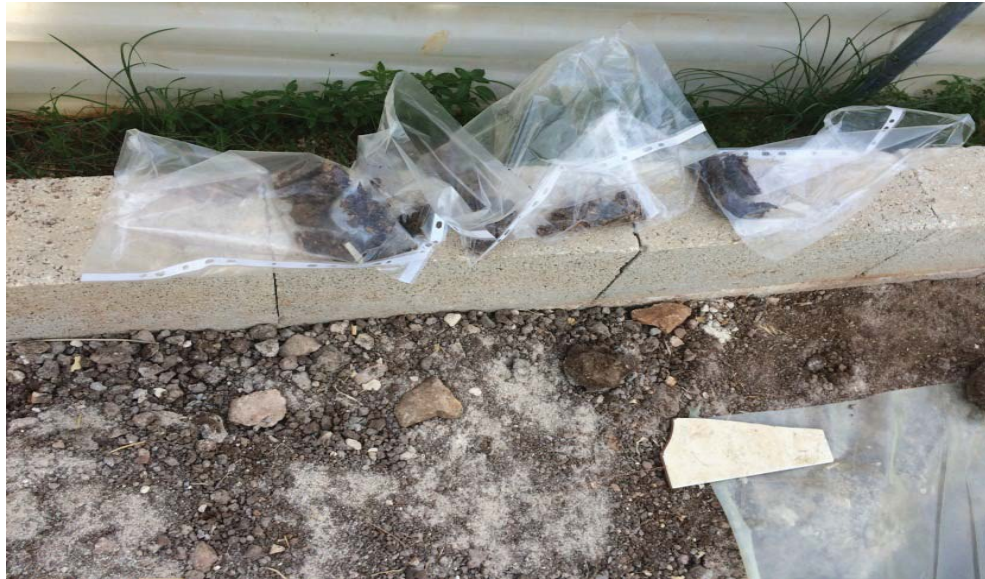
Sampling for PH and moisture content periodical tests
