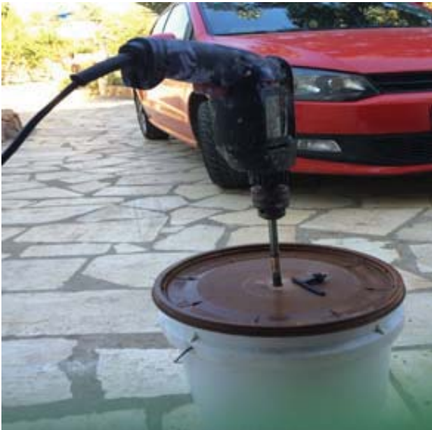
Assembled shredder along with starting the collection and shredding of organic materials
